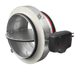
The CRS60 is a new circular fire damper with a fire resistance of up to 60 minutes. The optimised design of this fire damper (thinnest blade in the market) ensures excellent aeraulic and acoustic performance. A very compact collar and short damper tunnel (210mm) allow quick and easy mounting, both on-wall and remote. The new CRS60 damper is available in diameters 100-630mm.
